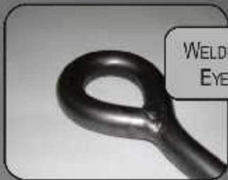
BARE A-36 STEEL BEFORE GALVANIZING
